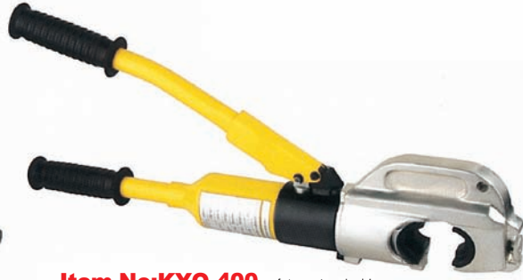
Item No:KYQ-400 safety system inside crimping range: 50–400mm 2 crimping force: 20T crimping type: hexagon crimping stroke: 25mm length: approx.540mm, weight: approx.8.30kg package: plastic box or steel case weight of case: approx. 4.00kg Accessories: crimping dies: 50, 70, 95, 120, 150, 185, 240, 300, 400mm 2
