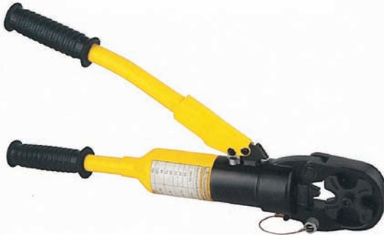
Item No:KDG-150 safety system inside open crimping head, rotate the die to choose crimping size. crimping range: 16–150mm 2 crimping force: 16T crimping type: indent crimping stroke: 20mm length: approx.500mm, weight: approx.4.60kg package: steel case weight of case: approx. 3.00kg Accessories: Female dies: 16, 25, 35, 50, 70, 95, 120, 150 mm 2 Male dies: 16–25–35, 50–70–95, 120–150mm 2
