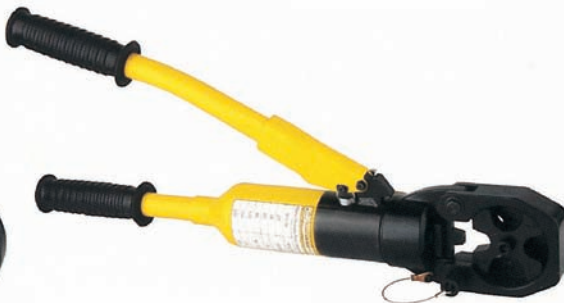
Item No:KDG-200 open crimping head, rotate the die to choose crimping size. crimping range: 16–200mm 2 crimping force: 16T crimping type: indent crimping stroke: 20mm length: approx.510mm, weight: approx.4.90kg package: steel case weight of case: approx. 3.00kg Accessories: Female dies: 16, 25, 35, 50, 70, 95, 120, 150, 185, 200 mm 2 Male dies: 16–25–35, 50–70–95, 120–150, 185–200mm 2
