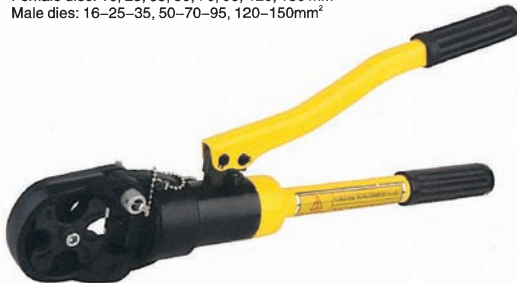
Item No:KDG-150A open crimping head, rotate the die to choose crimping size. crimping range: 16–150 mm 2 crimping force: 16T crimping type: indent crimping stroke: 20mm length: approx.470mm weight: approx.3.50kg package: steel case weight of case: approx. 3.00kg Accessories: Female dies: 16, 25, 35, 50, 70, 95, 120, 150 mm 2 Male dies: 16–25–35, 50–70–95, 120–150mm 2
