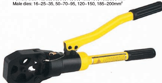
Item No:KDG-200A open crimping head, rotate the die to choose crimping size. crimping range: 16–200mm 2 crimping force: 16T crimping type: indent crimping stroke: 20mm length: approx.470mm, weight: approx.4.90kg package: steel case weight of case: approx. 3.00kg Accessories: Female dies: 16, 25, 35, 50, 70, 95, 120, 150, 185, 200 mm 2 Male dies: 16–25–35, 50–70–95, 120–150, 185–200mm 2
