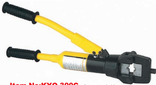
Item No:KYQ-300C safety system inside crimping range: 16–300mm 2 crimping force: 16T crimping type: hexagon crimping stroke: 20mm length: approx.500mm, weight: approx.6.80kg package: steel case weight of case: approx. 3.30kg Accessories: crimping dies: 16, 25, 35, 50, 70, 95, 120, 150, 185, 240, 300mm 2
